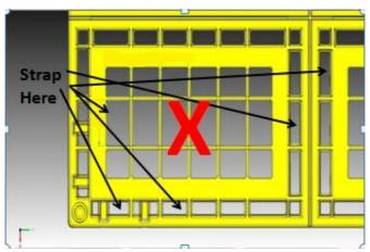
7.1.20 The cam/securing strap positions are located in the strongest parts of the panel.
