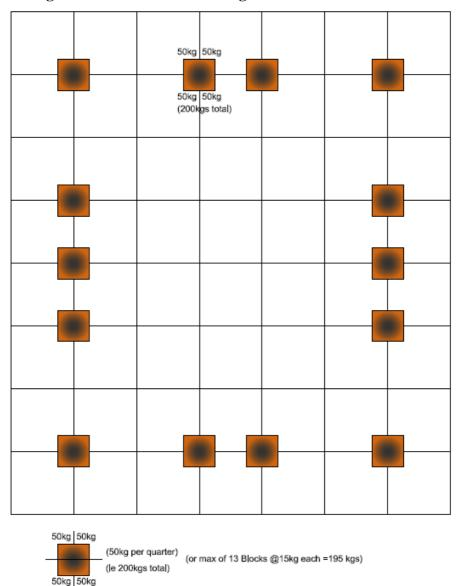
The above plan may overload a timber joist floor, as such we would advise this plan only to be used on the ground floor. In all cases the client must ensure the working surface can support the loads applied.
