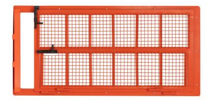
Where temporary void coverings are in place, such as would be used over a stair well. The principal contractor must ensure these are safe to access in-line with the Work at Height Regs 2005 Schedule 3 pt1. In addition, the cover must be designed in-line with the requirements of BS5975. Be installed by a competent person and handed over as complete and safe to access. Also, the cover must be visually inspected by a competent person daily to ensure it is safe.
