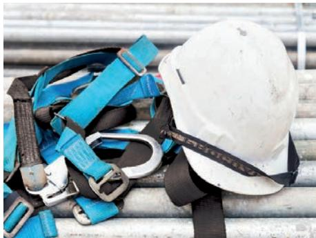
There is a wide range of possible damage to fall arrest/tool arrest equipment caused by misuse and abuse, general wear and tear, edge/surface damage, ultraviolet light, dirt, grit, chemicals and heat.
