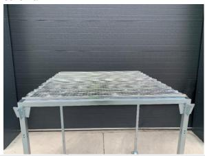
4. Insert two Leg braces diagonally on all corner bays. Leg braces are only required in bays at the corners of the system. Two braces are recommended as a minimum for each corner bay. When using make up panels this creates two separate systems so leg braces are required in the corners along the makeup panels.
