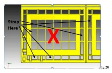
• The cam/securing strap positions are located in the strongest parts of the panel (fig 20)
