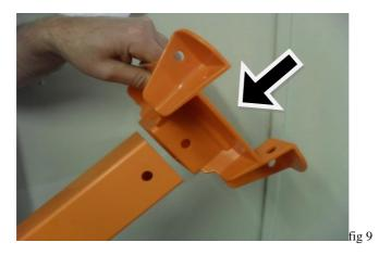
Put the securing pin through the pin holes securing the base & head plates to the leg.
