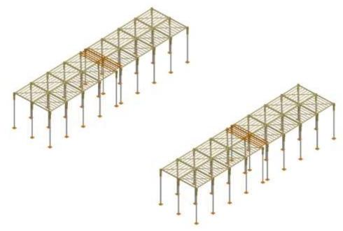
11. When completed proceed as above, alternating sides until the platform meets in the middle. If a gap is present, use infill units as described in Step 9.
