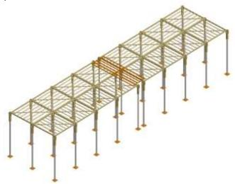
8. If the G-DECK platform requires extra rigidity, scaffold tubes can be fitted below using tubes and fitting to form leg bracing. If bracing below only fit where felt necessary to remove excessive movement.
