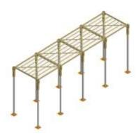
7. If the geometry dictates a gap in the centre of the run (see Step 8), lay an infill panel or deck panel over the gap and secure.
