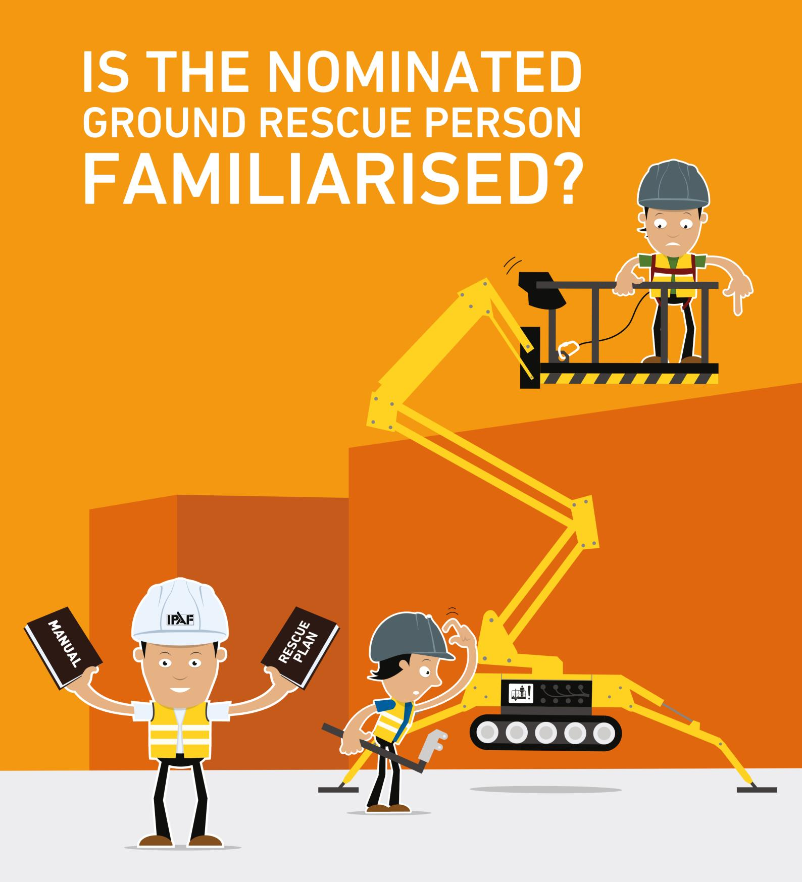
MEWPS ARE ALL DIFFERENT. LEARN AND PRACTICE THE GROUND CONTROLS AND THE AUXILIARY/EMERGENCY LOWERING CONTROLS AND PROCEDURES ON YOUR MACHINE.
