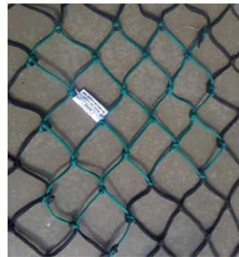
Figure 1. Permanent Repair to a Knotted Safety Net
