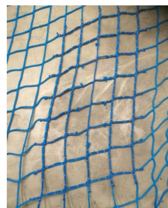
Figure 3. Permanent C Ring Patch Repair
