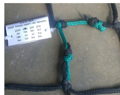
Figure 2. Permanent single strand repair to a Knotted Safety Net
