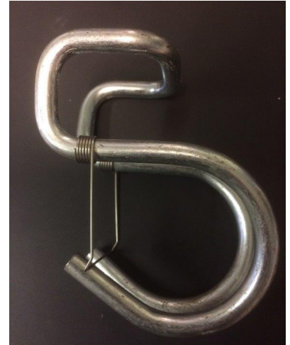
Figure 1. Example of spring modification to a safety net attachment device.
