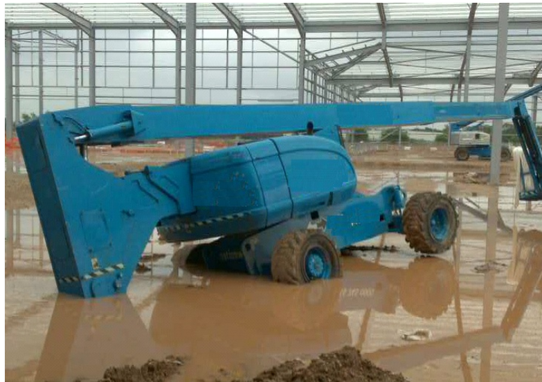
Figure 1. As an indication, a typical MEWP tyre or outrigger exerts a pressure of approximately 5 times that of a car tyre
