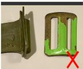
Figure 7, Left. Buckle deformed, sign of strain or result of a fall. DO NOT USE
