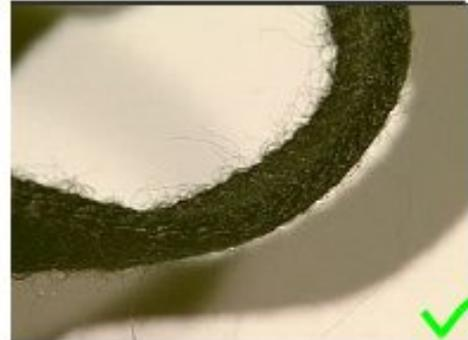
Figure 2, Right, webbing becoming 'Fluffy' sign of wear, to be monitored.
