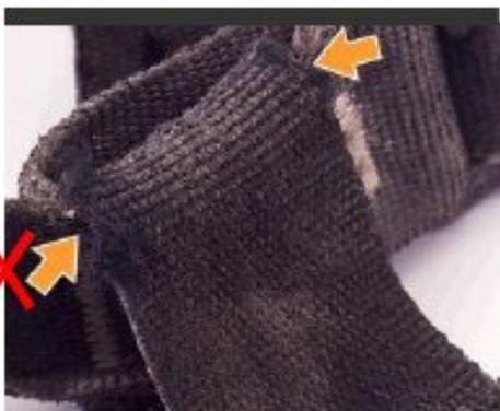
Figure 5, Left. Beginning of a break of at crossing point, refer to competent person for further examination
